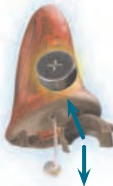
Remove the existing battery either by pushing it out the bottom of the door, or pulling it straight out.
